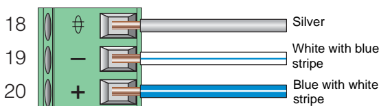
Figure 5–2: RS-485 connection
